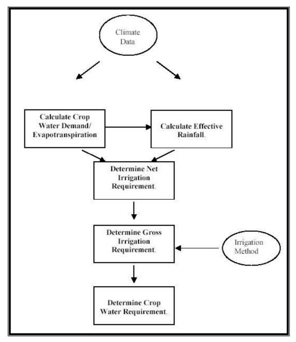
Figure 3.5 - Crop Water Requirement Determination Process
