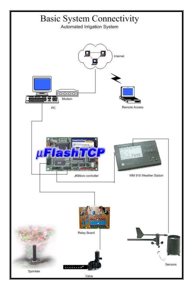
Figure 3.10 – Basic System Connectivity
