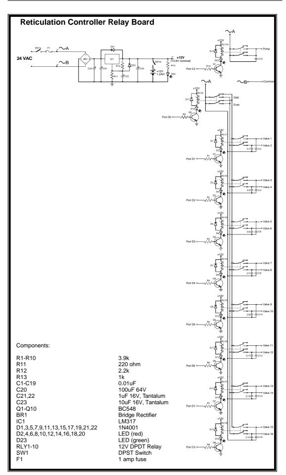
Figure 3.2 – Relay Board Schematic
