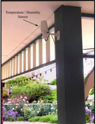
was securely fixed on top of the air conditioning unit, so it would be up high and out of the way of any debris that could fall into the unit. The anemometer / aerovane sensor unit was fixed to the existing television antennae pole. The temperature / humidity sensor (shown on the next page) was mounted underneath the back verandah of the residence, ensuring it would be not be in sunlight but
